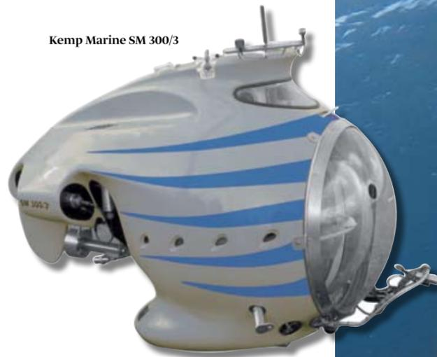
and submarine manufacturer Lamor Subsea for the private and leisure sector. Their SM 300/3 submersible is designed to dive to a depth of 300 metres whilst carrying two passengers in addition to the pilot. Buyers have options to customise the interiors and exteriors of
